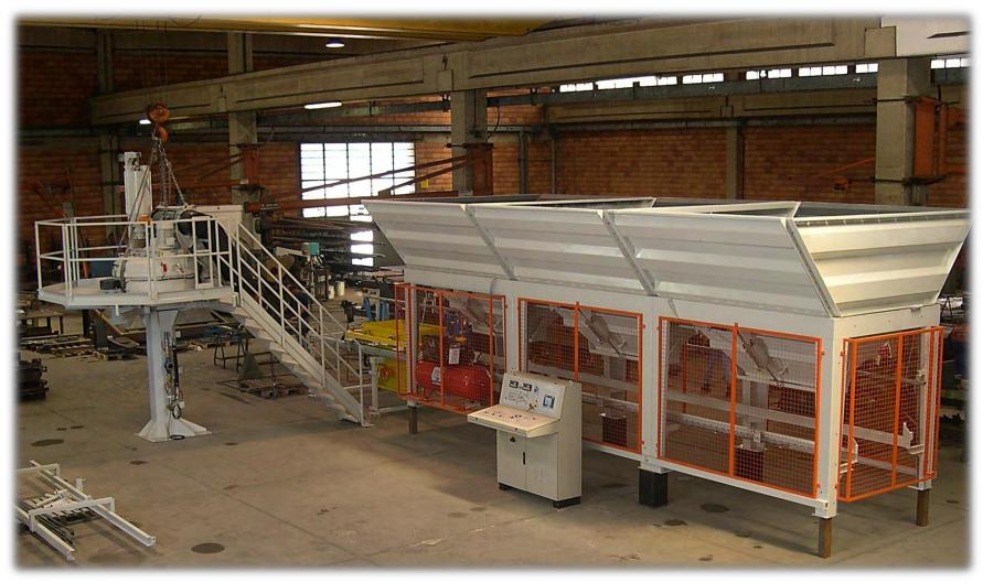
Pre-assembling inside works for Concrete Batching Plant manufactured by CM for a client in Manama, Kingdom of Bahrain
