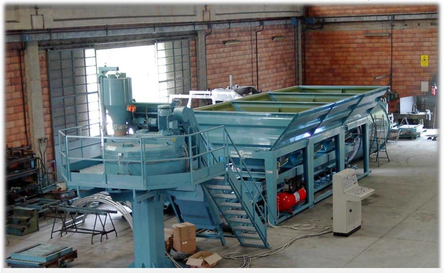
Each Concrete Batching Plant is tested inside works after pre-assembling made by CM for a client in Copiapò, Chile
