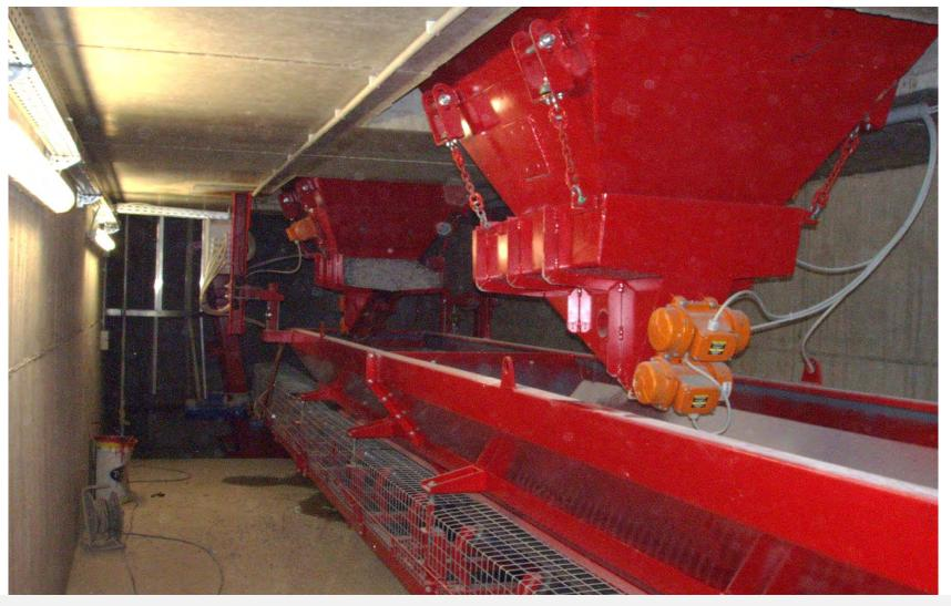
Concrete Batching Plant in Germany. Project and Machines manufactured by CM Aggregates dozing system made by weighing belt positioned at 5,5м underground quote ±0
